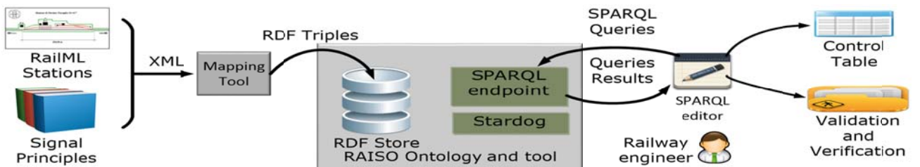
Figure 2: RAISO System Architecture for Railway Verification and Validation
